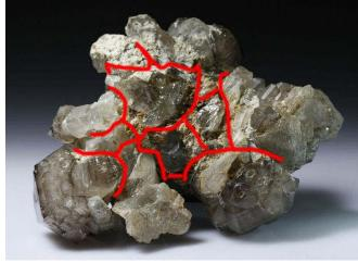
Above is the backside of fake specimen – the red lines indicate the areas where the glue composition is attaching all the lose crystals.
